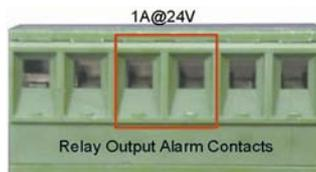
2. Verify that your load is wired to the central two terminals of this terminal block. After the relay is wired, insert this terminal block into its socket.
