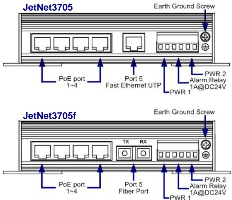
**To ensure the system working in a reliable status, please make sure it have make exactly grounding with Earth Ground Screw and System Earth Ground before powering.**
