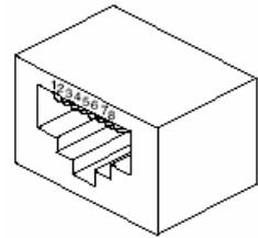
The following table shows the RJ-45 pin out for the PD.
