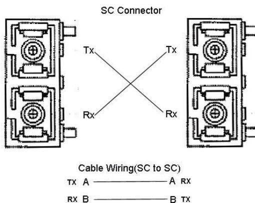
JetNet 3705f Series have one 100Base-FX port with SC type connector (in multi-mode and single mode versions). Single-mode types have greater distance capability than multi-mode types, but single mode cable is generally more expensive.
