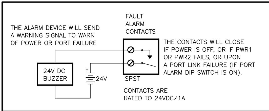
1. Connect to the SPST alarm relay terminals as per your application. Insert your load wires and tighten the alarm terminal screws to prevent the wires from coming loose. These contacts are open for normal operation and close in alarm. Do not exceed 24V and 1A current.
