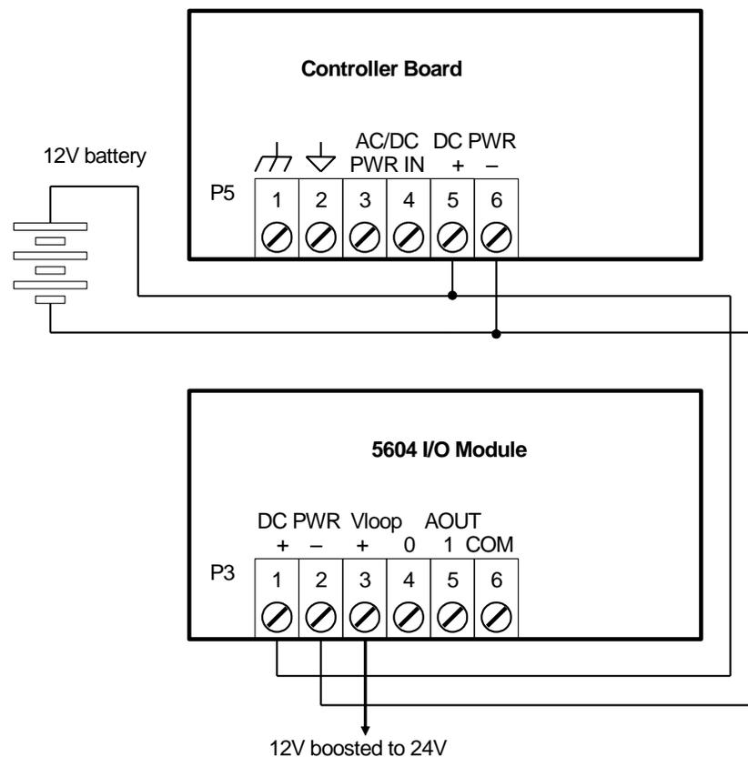
**Figure 4: Recommended Battery Configuration**
