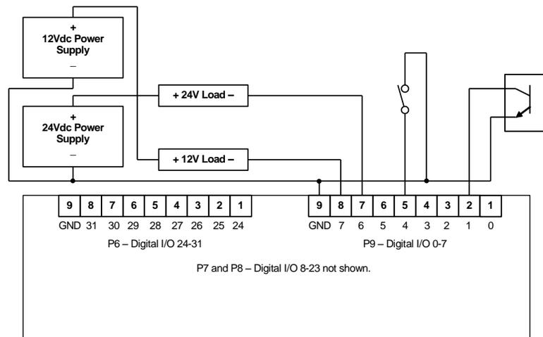
**Figure 10: Digital Input/ Output Wiring**
