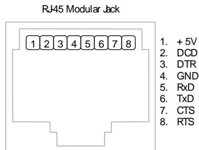
**Figure 11: Front View of an RJ-45 Connector**
