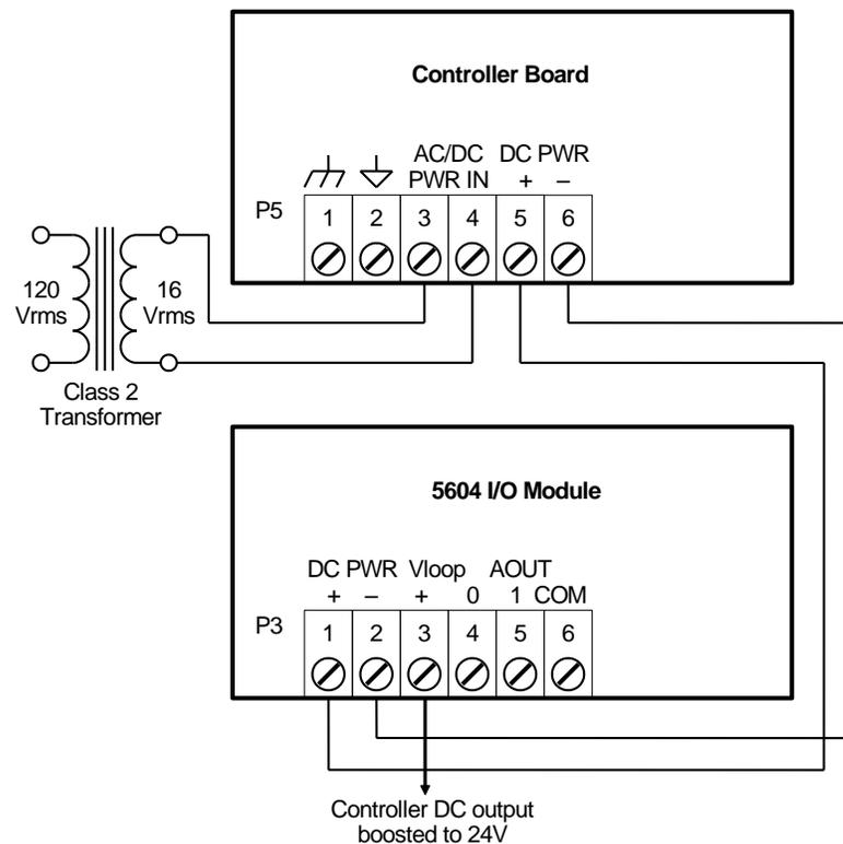
**Figure 2: Recommended AC Power Supply Configuration**
