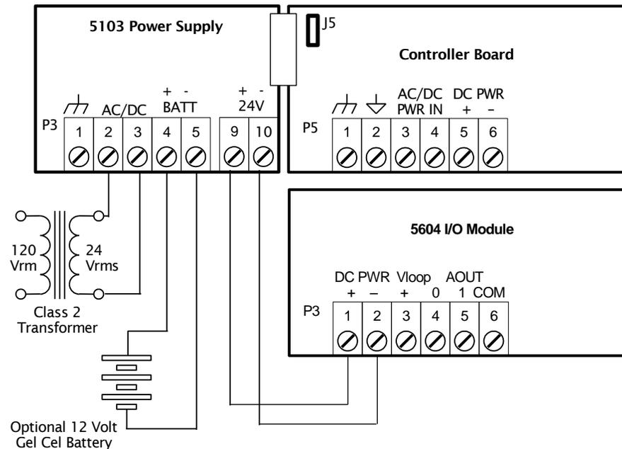
**Figure 5: Recommended 5103 Power Supply Configuration**
