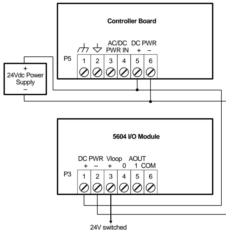
**Figure 3: Recommended 24V Power Supply Configuration**
