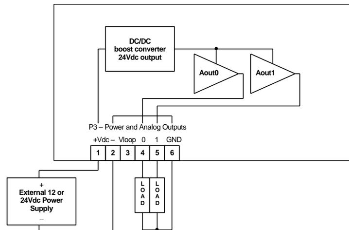
Figure 9: Analog Output Wiring
