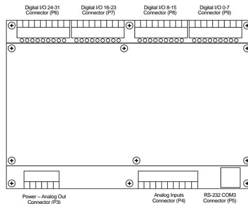
**Figure 1: 5604 I/O Module Layout**
