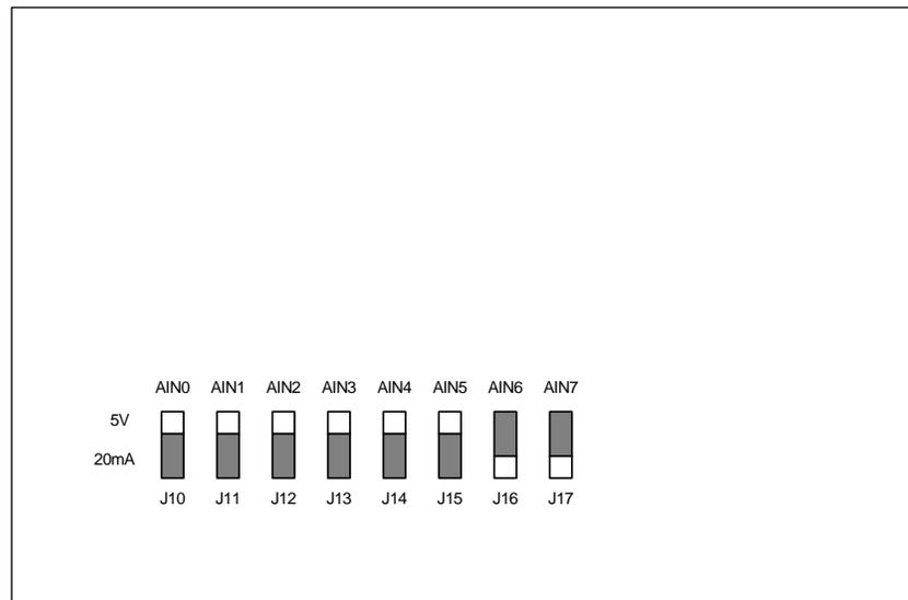
**Figure 7: Analog Input Mode Settings**
