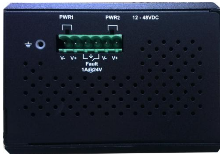
Figure-3: Top View of the PoE Injectors Industrial Switch
