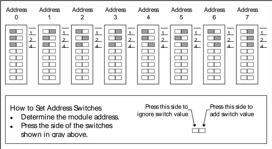
**Figure 4: Model 5403 Module Address Switches**
