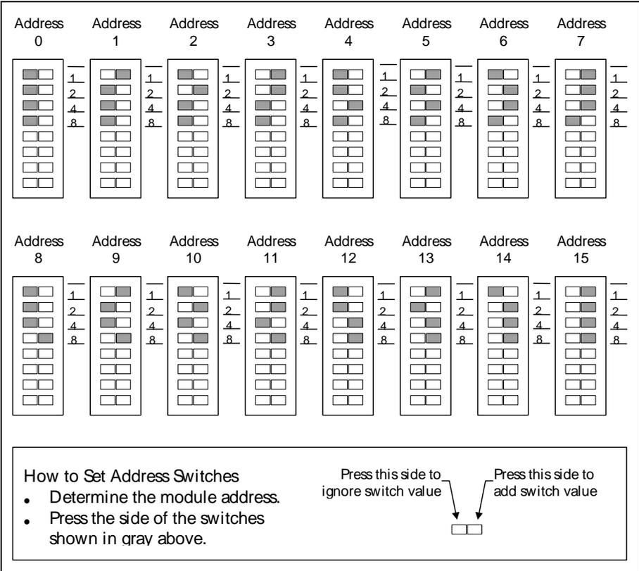
Figure 5: Model 5404 Module Address Switches
