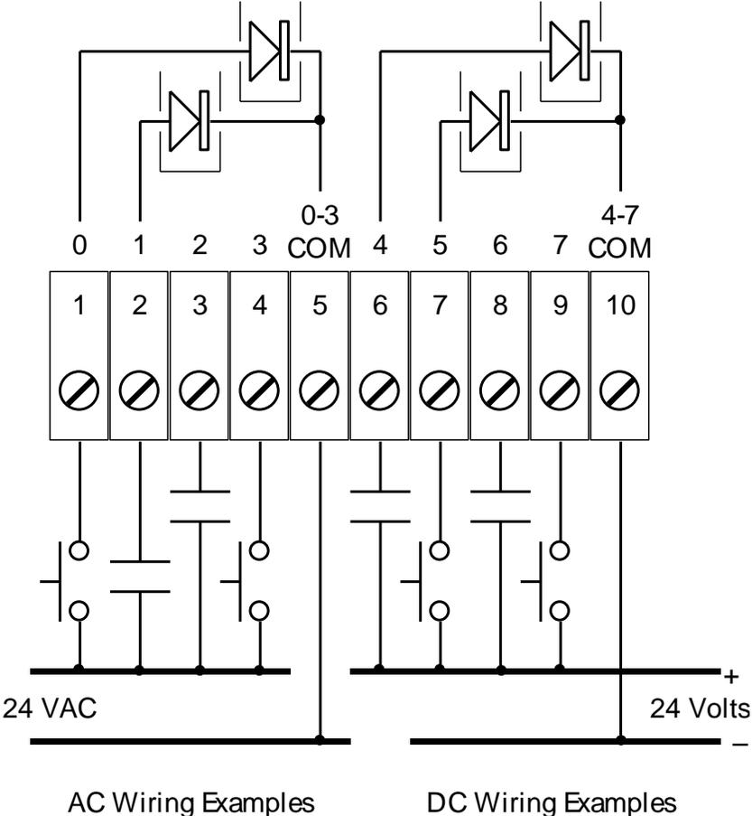
Figure 3: Field Wiring Examples
